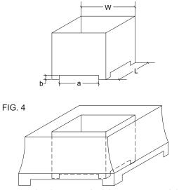
INTERNAL SHROUD REPRESENTS MINIMUM DIMENSIONAL DESIGN AND OPEN AREA (FROM FIG.4) THAT MUST BE PRESENT WHEN CONSTRUCTING SHROUD.
