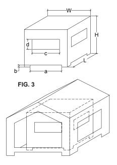
INTERNAL SHROUD REPRESENTS MINIMUM DIMENSIONAL DESIGN AND OPEN AREA (FROM FIG.3) THAT MUST BE PRESENT WHEN CONSTRUCTING SHROUD.
