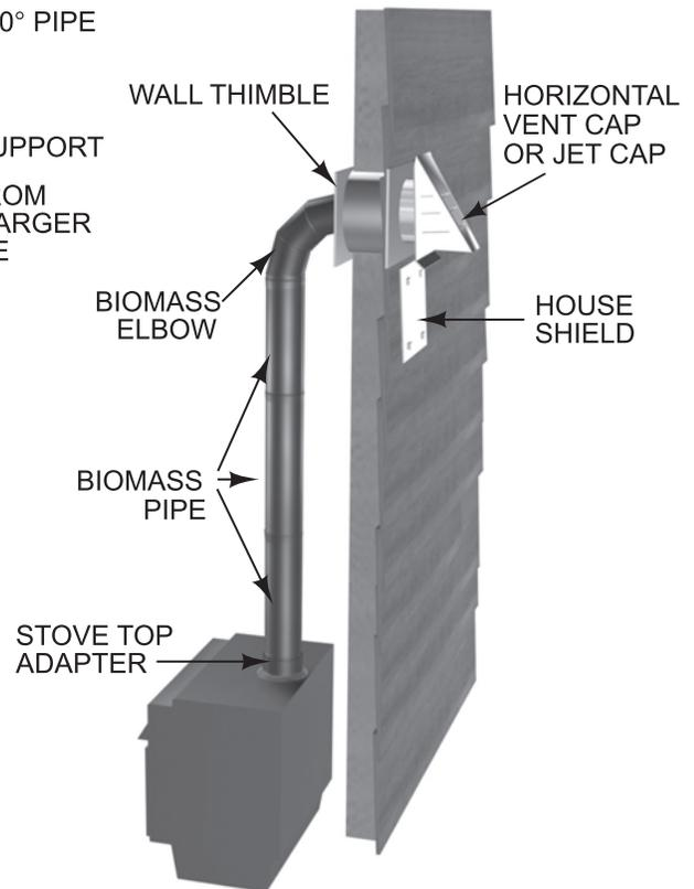
Note: Pipe overlaps 1 1/2" when joined together. Assembled length is 1 1/2" less than listed length.
