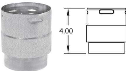
Use as a connector between stove exhaust collar and the positive twist lock of biomass chimney pipe. Order BSA when O.D. of exhaust collar is a true 3" or 4" dimension. Order BSAU when collar is less than 3" or 4" diameter.
