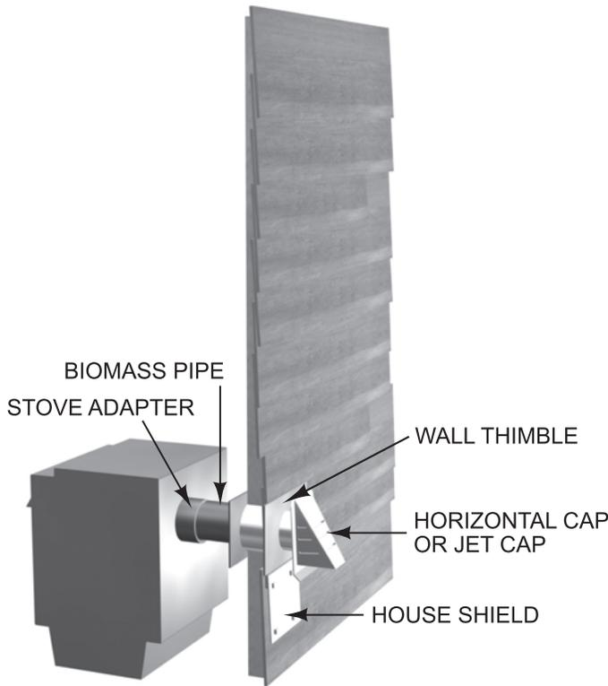
BIOMASS CHIMNEY REAR EXHAUST EXTERIOR - VERTICAL TERMINATION
