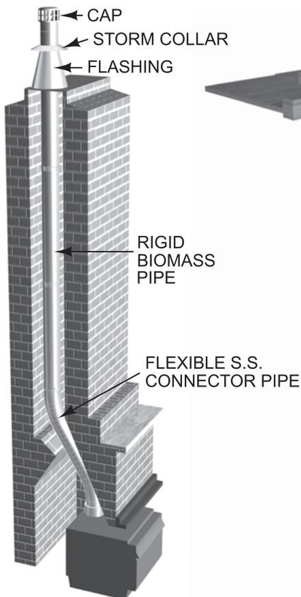
BIOMASS CHIMNEY TOP EXHAUST INTO EXISTING 2100° CHIMNEY
