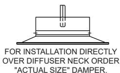
FOR INSTALLATION DIRECTLY OVER DIFFUSER NECK ORDER "ACTUAL SIZE" DAMPER.
