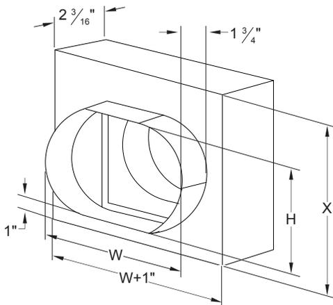
W = WIDTH (DUCT)      H = HEIGHT (DUCT)
