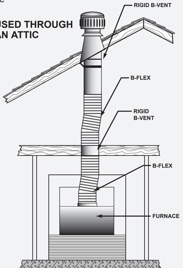
Easily connect furnace to termination on conventional installations.
