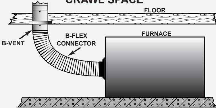
Easily connect furnace located in a crawl space to rigid B-Vent penetration.
