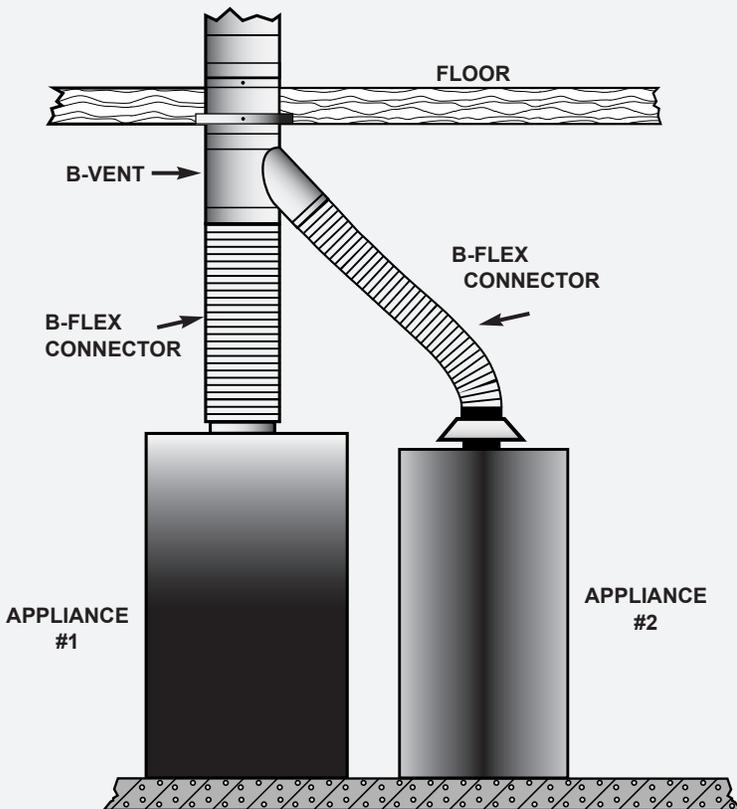
Make direct connection from one or both appliances to common B-Vent.
