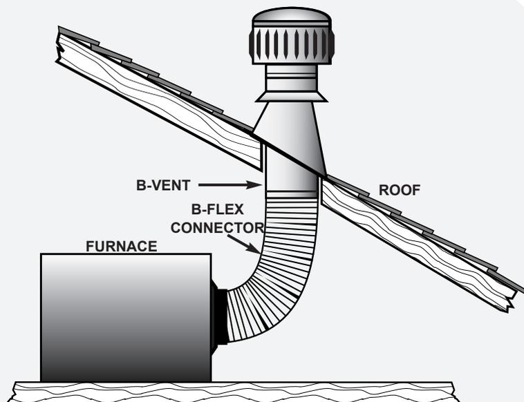
Make quick connection from attic furnace to rigid B-Vent penetration.
