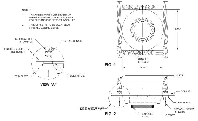
**NOTE:** The offset in the bowl is designed to come to the level of the finished ceiling. The trim will meet this offset. (See **FIG. 1** and **FIG. 2**.)
