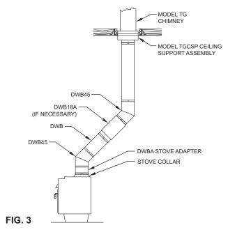
• If your stove has a rear outlet and you need to go upward, the Double Wall Black Tee (DWBT) can be used. A DWBA must be installed at the stove collar before attaching the DWBT. The DWBT then is installed onto the DWBA. If the listed chimney system is in a chase, and the DWB connector pipe must go horizontally, a Double Wall Black 90 degree elbow (DWB90) can be used. (See **FIG. 4**). Secure all joints with sheet metal screws.
