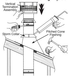
**Vertical Termination –** Align and press the vertical termination assembly down onto the vent pipe. Completely seat and secure the connection per the joint assembly instructions.
