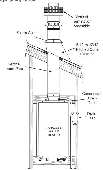
This kit can be extended up to the maximum allowable lengths as listed in the Use and Care Manual provided with the water heater. NOTICE: If a vent length of more that two (2) feet straight up from the top of the water heater is needed, a condensate drain line must be connected at the water heater.
