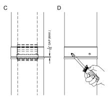
**Vertical Pipe –** Attach a length of pipe to the top of the water heater, completely seat and secure the connection per the joint assembly instructions.
