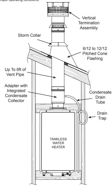
This kit can be extended up to the maximum allowable lengths as listed in the Use and Care Manual provided with the water heater. NOTICE: If a vent length of more that two (2) feet straight up from the top of the water heater is needed, a condensate collector must be installed at the water heater.
