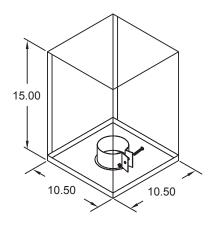
For use on open beamed pitched roofs or ceilings. Includes trim pieces for finishing out installation. Also includes support band.
