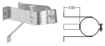
Provides exterior, vertical/lateral support for chimney. Maxiumum height of chimney which can be supported is 30 feet.
