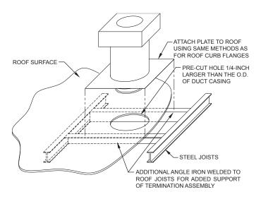
Once adequate support is available, install Fan / Curb Termination onto roof surface. The Fan / Curb Termination might require shimming in order to be level on the mounting surface. Attach Fan / Curb Termination plate to roof surface using similar methods used to secure roof curb to roof surface. Final sealing of roof surface should be applied after Fan / Curb Termination is installed or additional sealing of penetration will be required, as normally required for roof curb installations.
