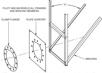
"X" is a minimum of 30° when bracing is used. A welded frame must be adequately attached to structural member for framework rigidity if bracing isn't used.
