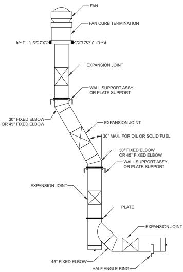
Bracing, above and below the elbows, is needed to avoid subjecting them to bending moments. In order for bracing to be effective, it must be rigidly attached to building members or foundation. The design of the structure used to attach supports must include the weight of the sloped section and whatever additional pipe is carried by the support. Additionally, an expansion joint is needed between the elbows to relieve thermal expansion stresses.
