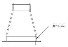
When ordering a square to round adapter, the size of the square end, flange requirements and diameter of the round end must be specified.
