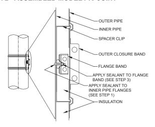
NOTE: Do not attach outer band with sheet metal screws through outer casing. Sheet metal screws could penetrate inner lining which could cause leakage, corrosion and expansion failure.
