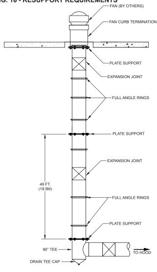
A plate support assembly is to be attached only to non-combustible construction such as block, concrete or steel with clearance that is adequate for installation and access.
