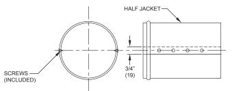
NOTE: Do not screw through casing of adjacent pipe.
