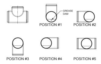
When a duct over 20" (508) diameter is used, a reduced tap 90° manifold tee may be used in lieu of the grease tee. Note that the tap must be at least 20" (508) in diameter.
