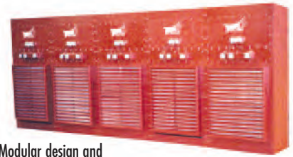
Modular design and multiple power modules allow the Clean Air Booth to meet specific needs.
