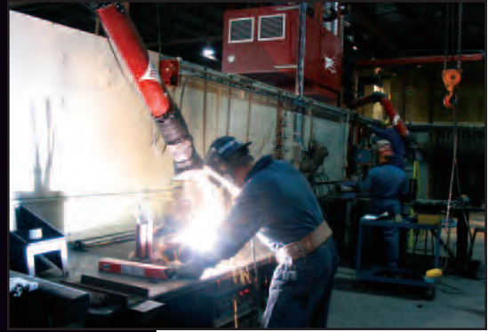
Source Capture of Weld Smoke and Fumes
