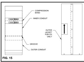
WARNING: Variable Length sections are not intended to be subjected to vertical force loads. Use appropriate support methods
