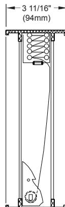
**Model MDFD3:** Metal-Fab Dynamic Fire Damper; 3-11/16" wide; 3-hour rating; dynamic airflow.
