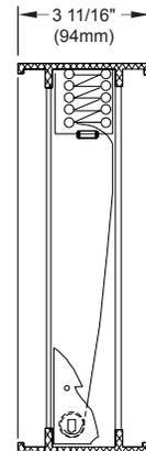
**Model MFDS:** Metal-Fab Fire Damper; slim-frame 2-3/16" wide; 1.5-hour rating; static airflow.
