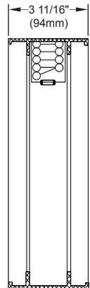
**Model MFD3:** Metal-Fab Fire Damper; 3-11/16" wide; 3-hour rating; static airflow.
