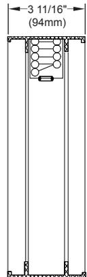
**Model MDFD:** Metal-Fab Dynamic Fire Damper, 3-11/16" wide; 1.5-hour rating; dynamic airflow.
