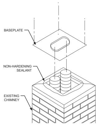
NOTE: Verify that there is sufficient room to mount the baseplate on to the masonry. You must have a level surface in order to install the baseplate properly.
