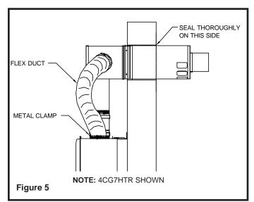
11. Using a general purpose silicone sealant approved for outdoor use, apply an adequate bead of sealant around the vent and exterior of the home. Failure to properly seal this wall penetration will result in long term damage due to weather conditions. (See **Figure 5**).
