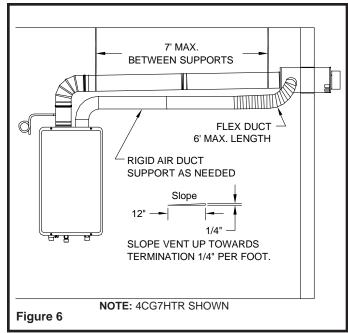
As previously noted be sure to seal penetrations with a general purpose silicone sealant approved for outdoor use. Failure to properly seal this penetration will result in long term damage due to weather conditions. Support venting lengths as per the manufacturer's installation instructions. Provide proper venting slope for horizontal venting and adequate measures to capture and dispose of condensate resulting from extended lengths of venting.
