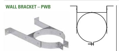
Used to provide lateral support while maintaining proper clearance. Recommended spacing is 6 ft. between bands above the starting point.
