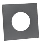
Used when pipe is supported by the TGAS. The oval I.D. of this plate covers any gap left between the chimney pipe and the ceiling. Select the plate which corresponds with the ceiling pitch. I.D. sized to fit over trim sleeve (TGTS).
